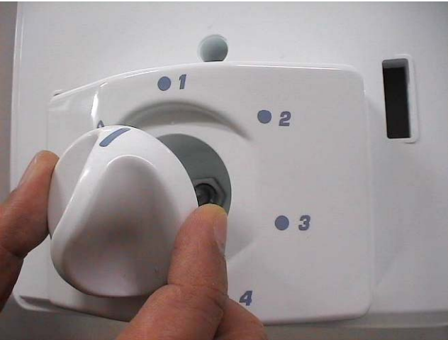
Slightly pull the thermostat knob towards you.
