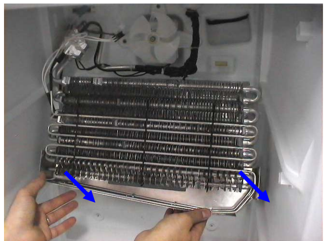
Disconnect to evaporator connector. (blue connector) Remove the evaporator by pulling forward in a horizontal direction. Do not push it up or down. You may break the fixing plastics.
